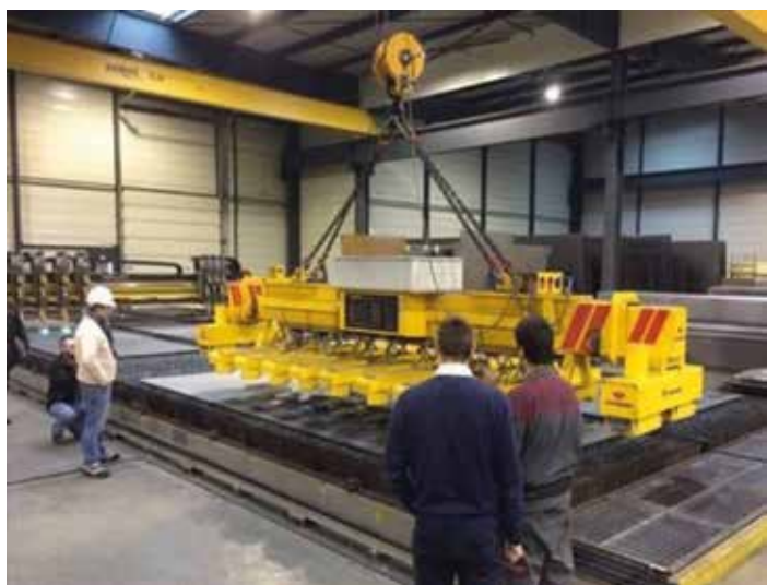
Permanent-electro COMBI series for loading/unloading cutting machines in a single operation (plasma, laser ...)
